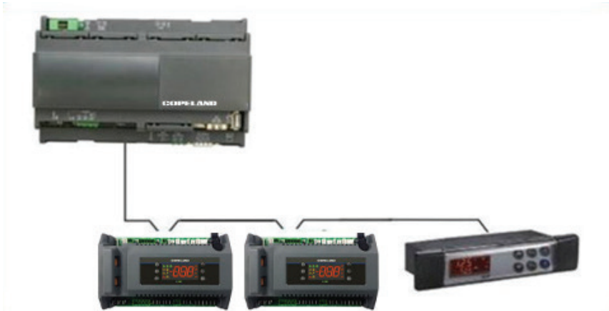
Figure 5. Correct network wiring
